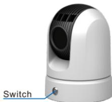
**[Notice] Switch/Indicator:** Long-press on the switch for 3 seconds to start the camera, then the indicator will be on all the time; when the camera is charging, the indicator will be on for 2.5s and off for 2.5s; when the battery is full, the indicator will be on permanently; when the battery lacks of electricity, the indicator flashes and be on for 200ms and off for 200ms.
